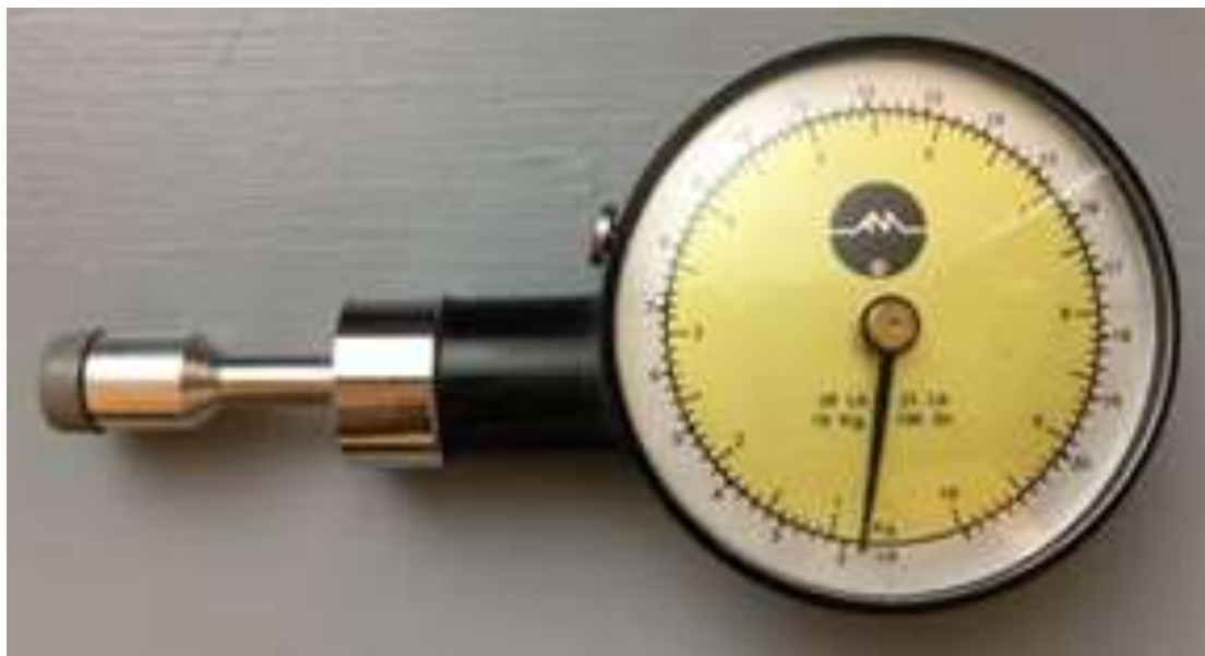
Figure 1. Algometer used to measure pain thresholds of tender and trigger points in test subjects with myofascial pain and fibromyalgia expressed in Kg/cm 2 . Equipped with a pressure distributing surface, it can be used to measure the amount of force performed by the test subject and is expressed in Kilograms.
